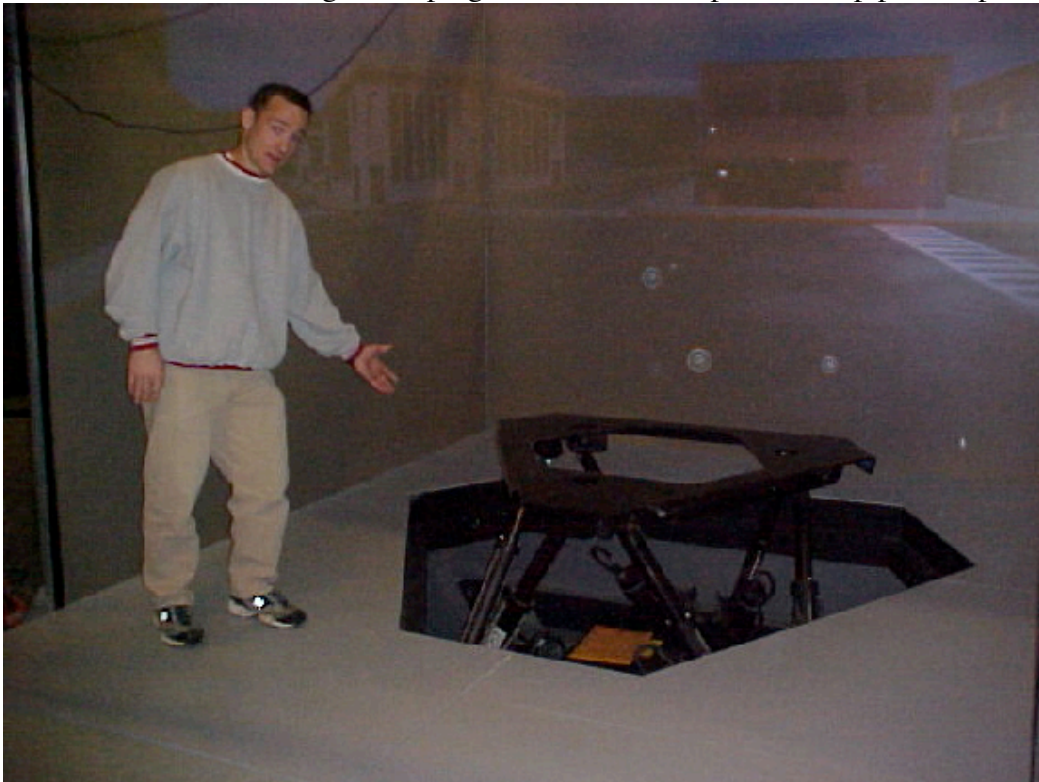
ACITC 3 rd floor: installing chair: plug removed motion platform top plate exposed
