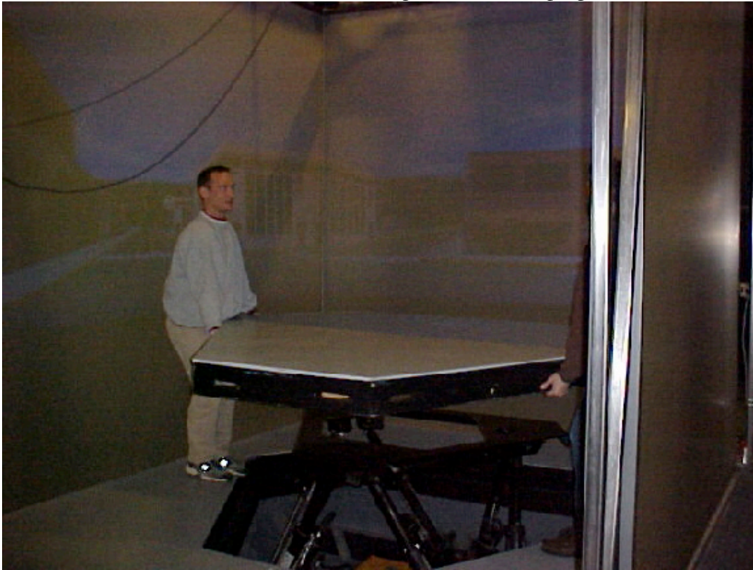
ACITC 3 rd floor: installing chair: plug removed motion platform top plate exposed
