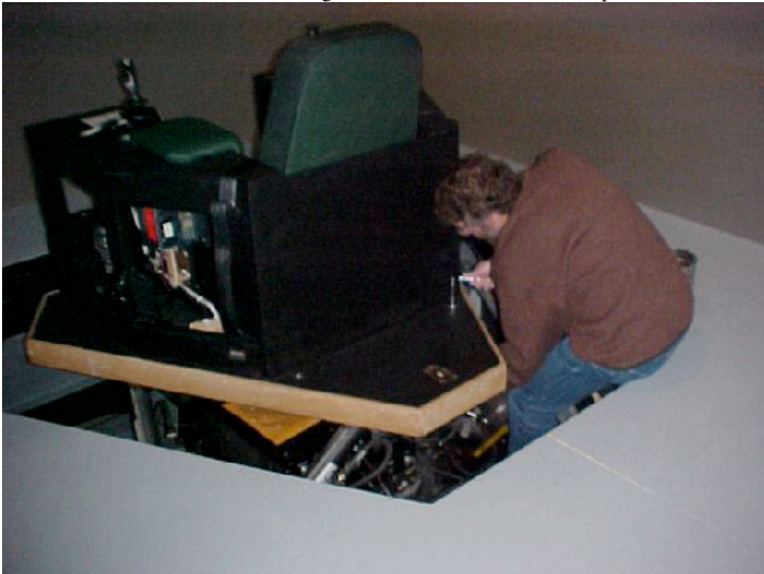
ACITC 3 rd floor: installing chair: bolt chair onto motion platform
